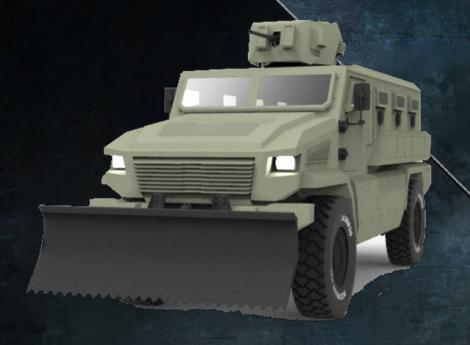
Designed for high mobility operations, both urban and rural, MRAP can carry a crew of 10, a driver and commander with 8 deployable dismounts. The vehicle is available with standard equipment such as run-flats, air conditioning and 2 point door locks. Optional equipment comprise of recovery winches, 360 deg turret, gunner stand,
